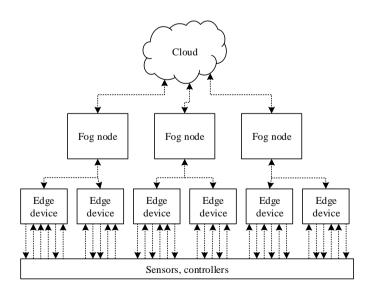
Figure 1. Hierarchical structure of the system using the cloud, fog and edge technologies
