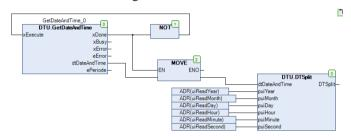
Figure 2. The program for reading the date and the time from the PLC
