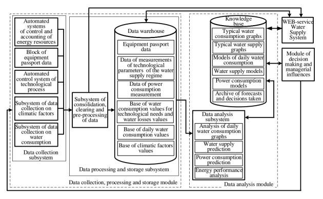
Figure 2. The architecture of operational control of energy efficiency modes of water supply facilities
