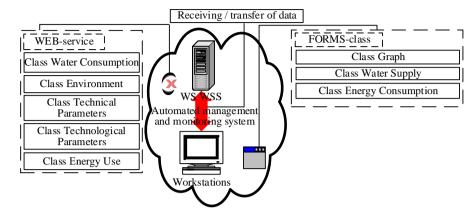
Figure 1. The architecture of operational control of energy efficiency modes of water supply facilities
