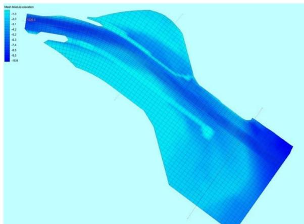
Figure 3. Bathymetric data over calculation grid
