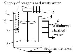
Figure 3. The scheme of the mixer-reactor of periodic action with mechanical stirring and with the function of settling: 1 - electric motor with gearbox; 2 - the housing of the mixer reactor; 3 - perforated protective tube; 4 - vertical plates; 5 - rods for fastening pH and Eh converters; 6 - pipelines for drainage of clarified water; 7 - pH and Eh converters; 8 - the blades of the mixer
