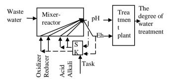
Figure 1. — Structural scheme of wastewater treatment with regulation of pH and Eh with the introduction of various reagents (SK - control system)
