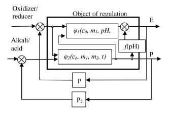
Figure. 2. Structural scheme of two-channel system of regulating the dosage of reagents: P<sub>1</sub> - regulator Eh; P<sub>2</sub> - regulator pH;  $\varphi_1$  - function of transforming redox process;  $\varphi_2$  - function of transformation of process of acidification; f(pH) - dependence Eh on pH;  $c_o$  - concentration of admixtures;  $m_1$  - mass of added reducer;  $m_2$  - mass of added acid; t - time
