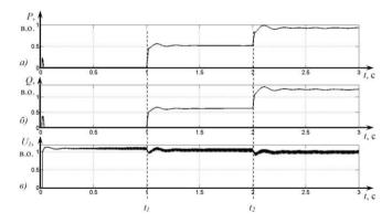
Figure 4. Graphs as a function of time t, showing the functioning of the hydrogenerator on the consumer active-inductive load: a) - active power of the generator P, r.u.;  $\beta$ ) - reactive power of generator Q, r.u.; B) - the current value of the voltage on the load U1, r.u.; t1 - moment of connection of load Load1 by Breaker3 switch; t2 - load connection time of Load2 by Breaker4 switch.
