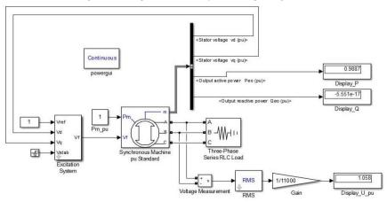
Figure 2. Structural scheme of a computer model of a synchronous generator, taking into account the presence of an excitation system
