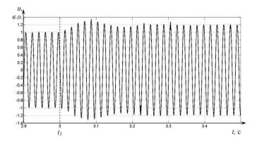
Figure 5. Instantaneous voltage values (in r.u.) on the consumer load of the hydrogenerator when increasing, by means of the excitation system of the synchronous machine, the value of the voltage of the generator from 1 r.u. up to 1,2 r.u. at the time of model time t3=3s.
