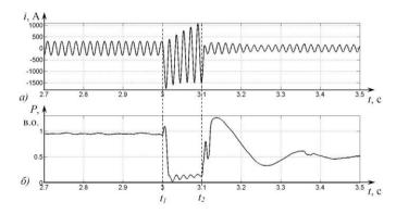
Figure 6. Graphs as a function of time t, characterizing the processes in the autonomous power system at three-phase short circuit in the load line of Load1:
